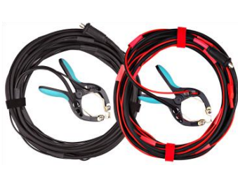
Current and Sense cables with TTA clamps
