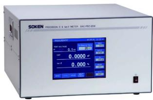
Introducing a current transformer type comparator bridge, DAC-PSC-20W gives automatically Capacitance and Dissipation Power Factor tan delta in a comparative measurement of a specimen and standard capacitor.
