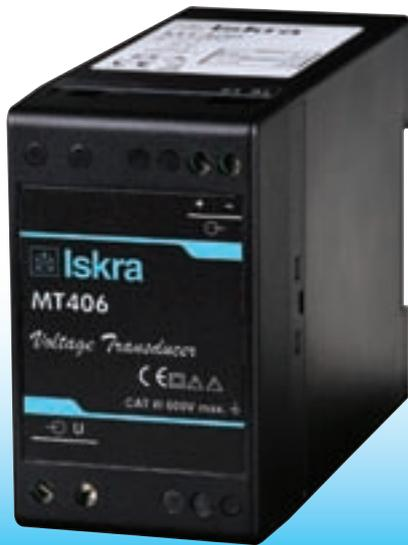
MT406 is intended for measuring and monitoring voltage in electrical power network. Voltage input is electrically insulated from the system by means of voltage transformer. The signal is rectified, smoothed and amplified into an independent DC current output.
