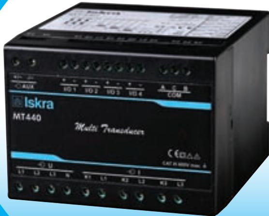
MT440 are intended for measuring and monitoring single-phase or three-phase electrical power network. They measure RMS value by means of fast sampling of voltage and current signals, which makes instruments suitable for acquisition of transient events. A built-in microcontroller calculates measurands (voltage, current, frequency, energy, power, power factor, THD phase angles, etc.) from the measured signals.
