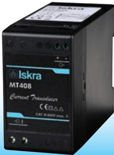
MT408 is intended for measuring and monitoring single-phase electrical power network. Current input is electrically insulated from the system by means of current transformer. The signal is rectified, smoothed and amplified into an independent DC current output.
