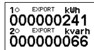
Picture 12: Examples of presented data on graphic LCD
