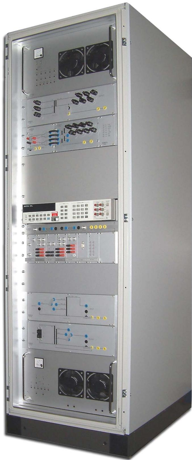
The new ZERA single phase precision power calibration system PPCS is developed for the traceable calibration of measuring instruments for active-, reactive and apparent power and has a great importance for national metrology institutes.
