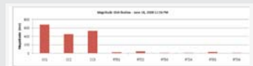
Figure 2 High PD levels at Capacitors. Low PD levels at RTD’s.
